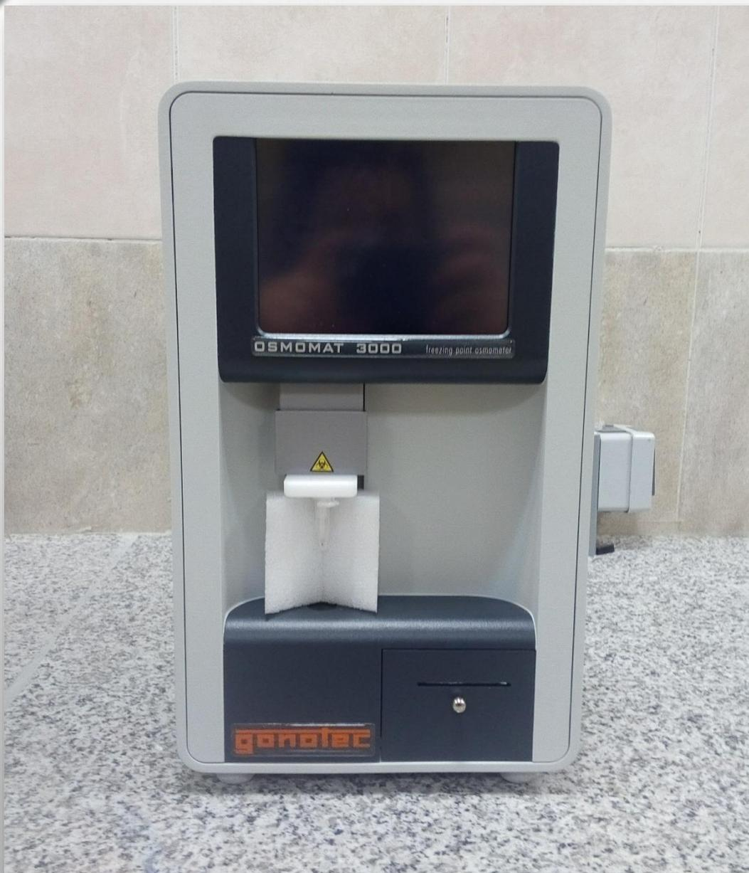
An Osmometer is a scientific instrument used to **measure the osmolality of a liquid sample**, which indicates the concentration of solutes present. It finds applications in fields such as clinical diagnostics, pharmaceuticals, and research laboratories, enabling the assessment of fluid balance, determination of osmotic pressure, and quality control of solutions in various industries including healthcare, biotechnology, and food and beverage.
