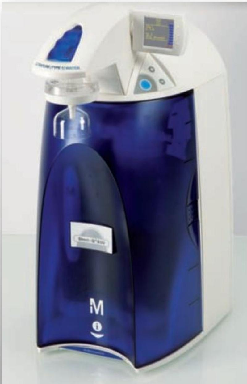
An Ultra Pure Water Generator is a device that produces **high-quality water** with **extremely low levels of impurities** and **contaminants**. It finds applications in fields such as pharmaceutical manufacturing, semiconductor fabrication, laboratory research, and healthcare facilities, providing a reliable source of ultrapure water for critical processes like analytical testing, equipment cleaning, and sensitive experiments requiring water of exceptional purity.
