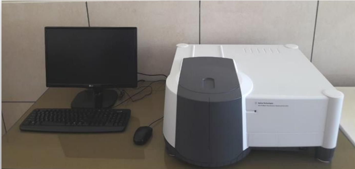
Fluorescence Spectroscopy is a powerful analytical technique that **measures the emission of fluorescent light** from a sample upon excitation with specific wavelengths. It finds applications in fields such as biochemistry, pharmaceuticals, environmental monitoring, and material science, enabling the study of molecular interactions, protein folding, cellular imaging, and **detection of pollutants** or **biomarkers** with high sensitivity and specificity.
